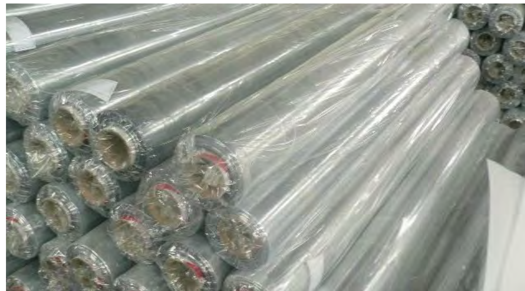
(above) PVC rolls produced by calendaring.
