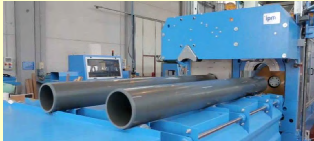
PVC Pipe created using extrusion process
