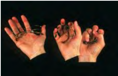
Shape Memory Alloy used in spectacle frames
